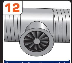
Turn on air handlers and fans once the finish has started to dry to assist in the drying/curing process.
