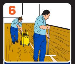
Pour a 3"- 4" wide strip down the length of the gym to the opposite corner while pulling your applicator through the finish. Continue back and forth down the floor, pouring additional beads of finish as needed.
