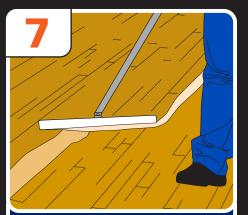
Overlap 4 to 6 inches. Pour finish onto the floor from behind the applicator during each full length pass. Angle the applicator so finish runs off to the unfinished side. Do not allow a puddle to form in front of the applicator.
